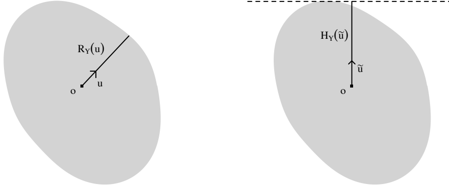
Figure 1.4: For the two-dimensional particles Y (grey), the radial function R_Y(u) in direction u (left) and the support function H_Y(\tilde{u}) in direction \tilde{u} along with the supporting hyperplane (dashed line) with normal vector \tilde{u} (right) are shown.
