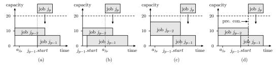
Figure 4. Scheduling the job  $j_p$ . The limiting constraints are: (a) The sequence, (b) time window, (c) capacity, (d) precedence constraint.
