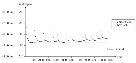
Figure 7. Makespan in minutes as a function of CPU time in seconds. A point is inserted after every 50 iterations of the algorithm.
